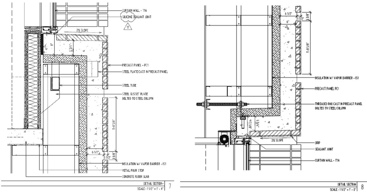
Figure 1: Precast Panel Connection Details
