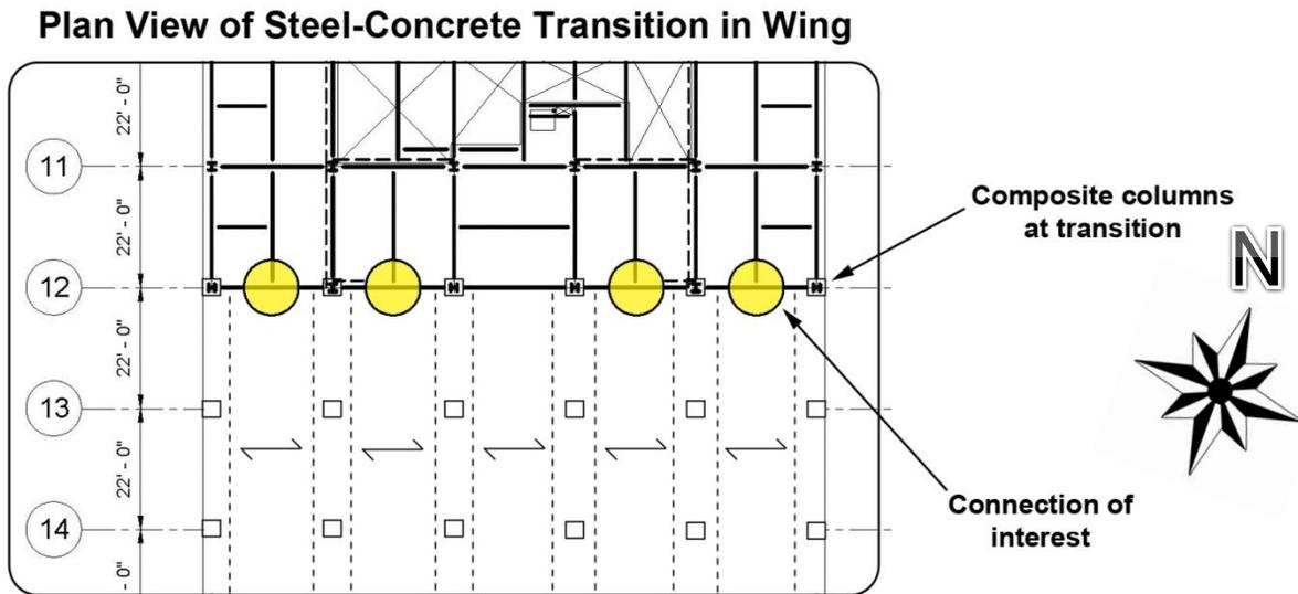
Figure 40: Transition at grid line 12
