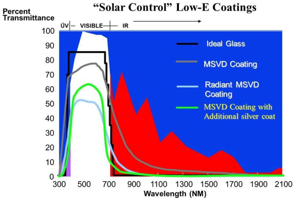
When compared to tinted or “moderate” spectrally selective glazing, the “solar control low-e” glazing more closely matches the ideal glass type transmission curve. The graphs for tinted and “moderate” spectrally selective glazing are shown below.
