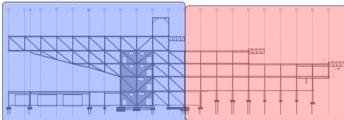
Figure 39: Division of the Steel and Concrete Systems.
