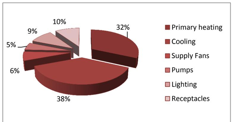
**Figure 17: Existing Energy Breakdown**
