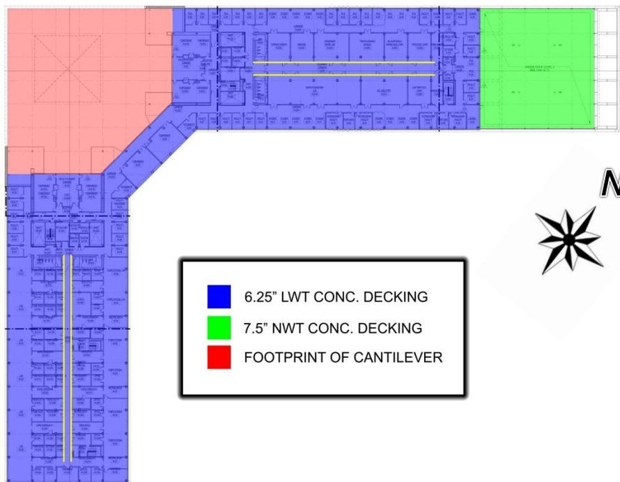
Figure 19: Typical Floor Layout
