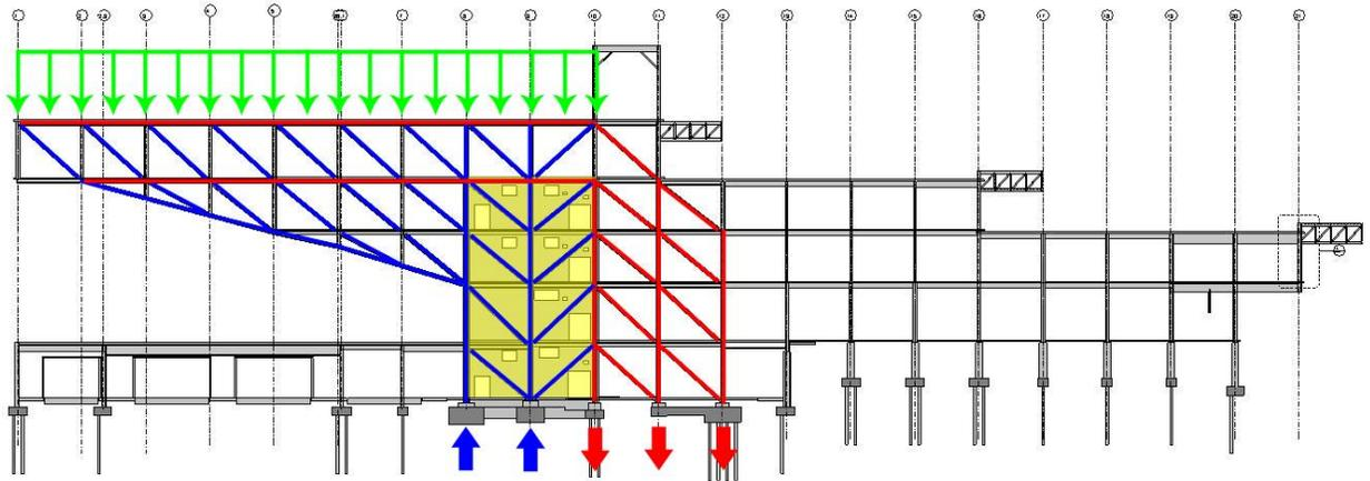
Figure 20: Special Systems load distribution
