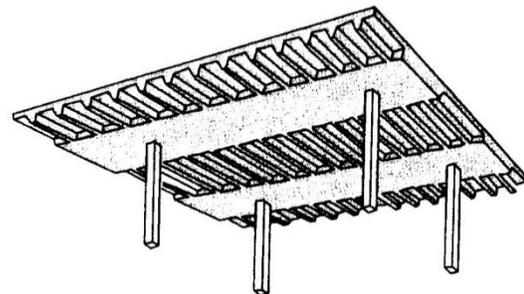
Figure 37: Pan Joists
